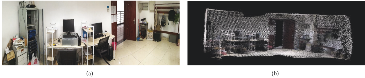
FIGURE 4: Recognition of multiobjects with SLAM algorithm: (a) real indoor scene and (b) reconstruction result with SLAM algorithm.
